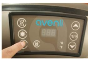
5) Connect the pump unit then press the button to inflate the spa. The air flow valve prevents your spa from over-inflating.
