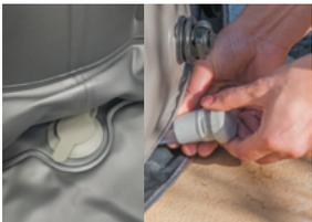
10) Ensure that the drain caps are properly closed before filling the spa
